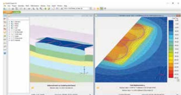
3D Finite element analysis to study the behaviour of two tank foundation
