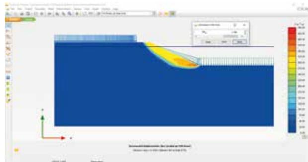
2D Finite element analysis for de evaluation of slope stability in embankments with soil improvement
