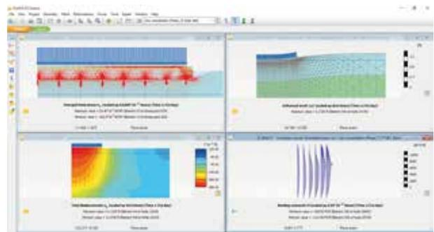
2D Finite element analysis for de evaluation of settlements and soil stresses
